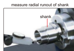
measure radial runout of shank
