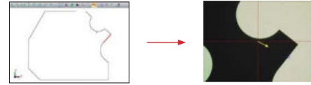
Input CAD drawing and set reference, move the stage to make the target box in the center of crosshair, then the software will do automatic measurement
